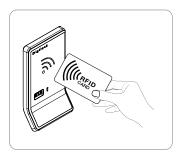
Unlock: Present an assigned User RFID credential.
